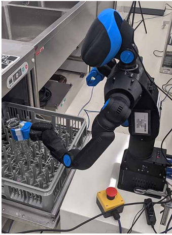
Fig. 2: A grasp of a transparent object performed by our robot using our network for point cloud depth completion.
